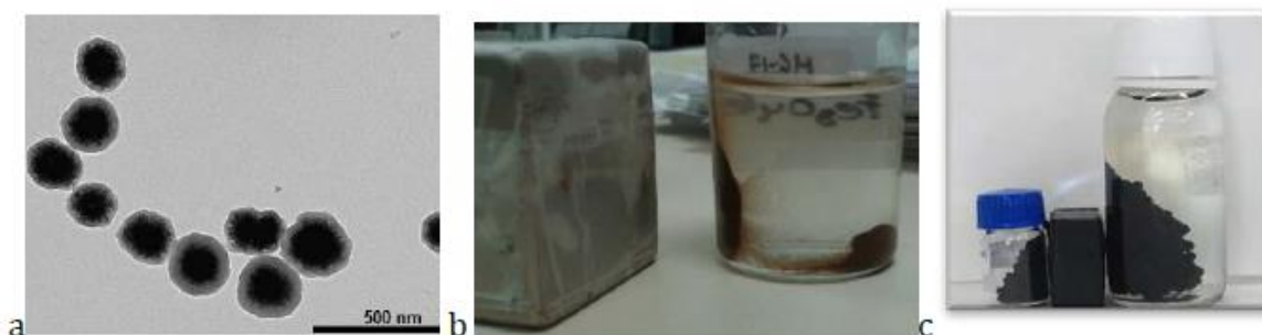
Figure 1. Magnetite coated with carbon (a) or aluminium hydroxide (b) and particles in the millimetre range composed of biopolymers, magnetite NPs and inorganic carbon, (c).
